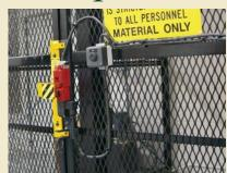
All Beech MATERIALIFT® VRCs meet the ANSI/ASME B20.1-2000 safety standard for conveyors. We can supply all required safety enclosures and gates with interlocks, as well as further safeguards (such as automatic load stops to contain off-balance or rolling loads). Just ask your Beech representative for further details. And remember: MATERIALIFT® VRCs are for material loads only!
